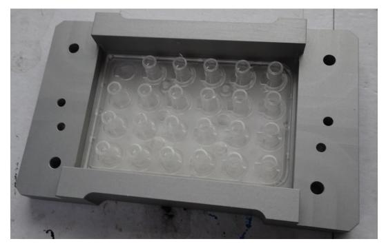
Turn electrode manifold (with handles as on page 5) upside down and place HP cover with Costar transwell plate on the electrode assembly:
