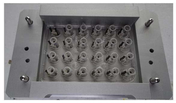
Check the position of the tip of the APICAL voltage electrode. The distance between tip of V-electrode and membrane should be at least 1 mm. See next page.
