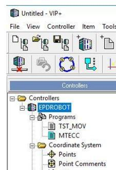
In the *Controller window* of VIP+: highlight the “*Controllers*” folder and hit the icon
