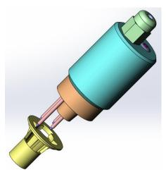
The conic shape of the upper part of the individual Costar wells is somewhat different from the shape of wells in the 24 well plates. In order to obtain a stable fitting we designed the lower part (in brown) of the IV electrode. The other parts (top, cable, etc...) are the same as those in EL-CSMW-SINGLE.
