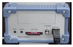
The unit is powered with a power bank which is commercially available (for tablets and mobile phones). Alternatively, power can be obtained from a PC (see switch PC/Local).
